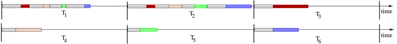
Figure 3: The N-way Basic Stream Combination Technique.
