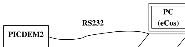
Figure 2: Part1 and Part2 are interconnected using RS232 serial communication
