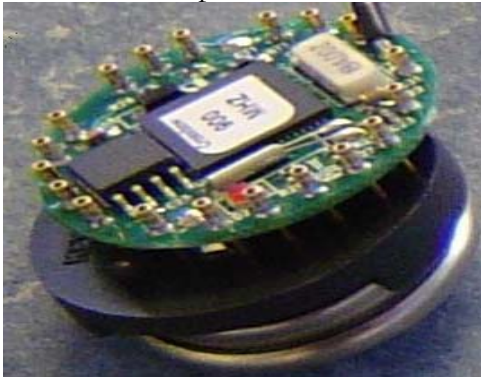
Figure 2. Wireless infrasonic sensor.
