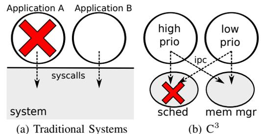
Fig. 1. (a) Traditional application-level, fault tolerance using a technique such as check-pointing or recovery blocks for recovery. (b)  $C^3$ : for the recovery of failed system services, within bounded time, and at the priority of any application that requires service.
