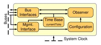
Figure 4: AIR Observer architecture
