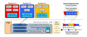
Figure 2: Two-level hierarchical scheduling with partition scheduling featuring mode-based schedules
