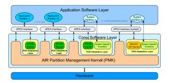
Figure 1: AIR architecture for TSP systems
