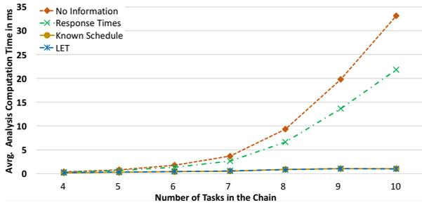
Figure 7: Average analysis time in cause-effect chains with 2 involved periods.
