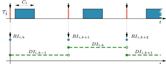
Figure 5: Read and data intervals of consecutive jobs of  $\tau_i$  if the system operates based on the LET model.
