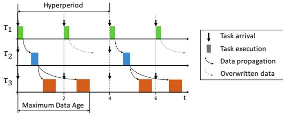
Figure 1: Data propagation between tasks of a cause-effect chain in a real-time system with maximum data age specified.
