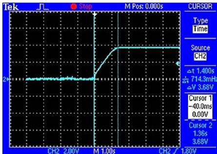
Figure 13: Charging time for a DC input. This dictates the preamble necessary at an input DC voltage of 3V, when the source and panel are apart by a distance of 21mm.
