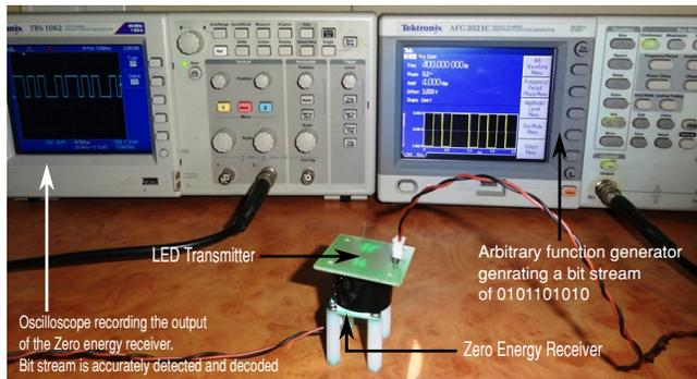
Figure 10: A view of the receiver decoding a random bit stream
