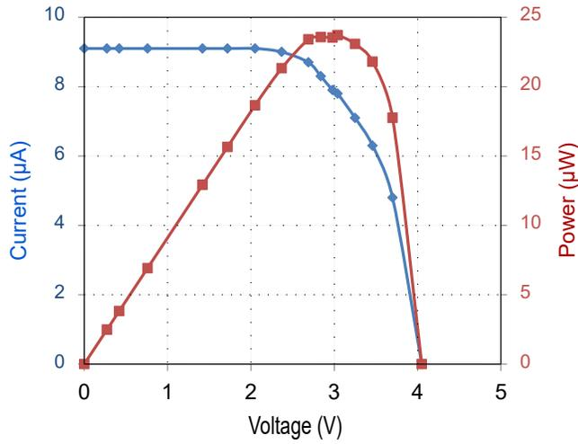
Figure 2: DC Characteristics of CPC1824 at 3000LUX
