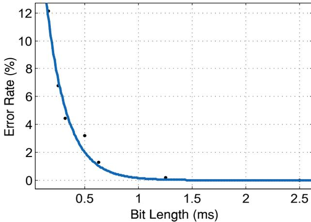
Figure 12: Bit error rate versus bit length
