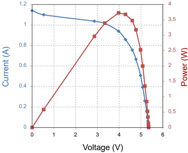
Figure 3: DC Characteristics of SP4.2-37 at 6150LUX
