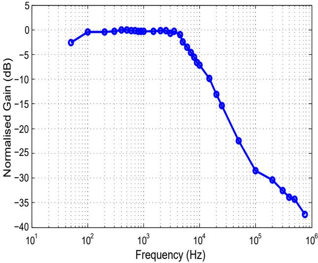
Figure 6: Frequency Response of SP4.2-37 for a  $C_0$  value of  $1\mu F$
