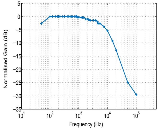
Figure 5: Frequency Response of CPC1824 for a  $C_0$  value of  $1\mu F$
