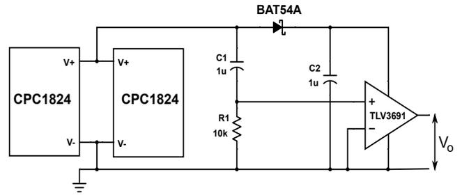
Figure 8: Receiver with the comparator connected
