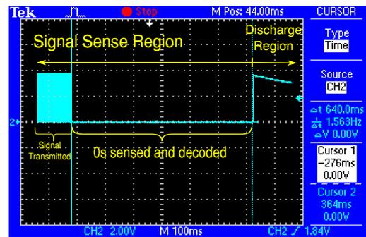
Figure 15: Response of the system when a continuous stream of 0s are transmitted. A maximum duration of 640ms can be tolerated by the system. This is independent of the bit length
