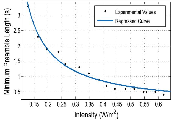
Figure 14: Dependence of preamble length on light intensity
