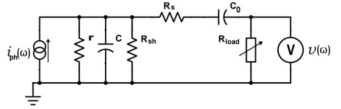
Figure 4: Equivalent Circuit model for AC signals
