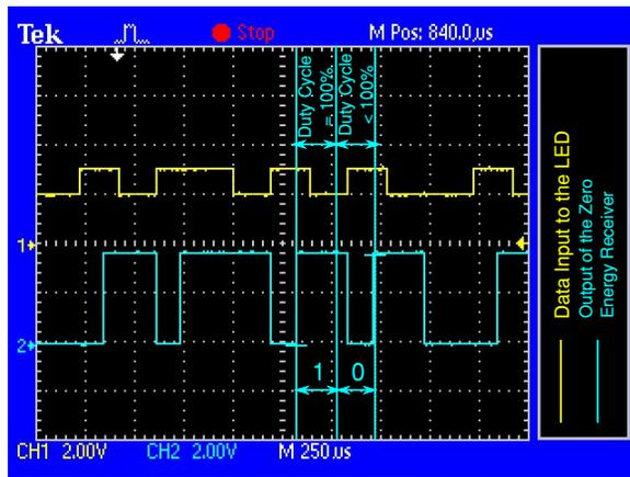
Figure 16: Duty Cycle approach to decode high data rates
