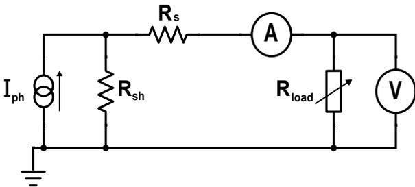
Figure 1: Equivalent DC model of the solar panel
