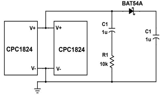
Figure 7: High pass filter and peak detector cascaded with the panels
