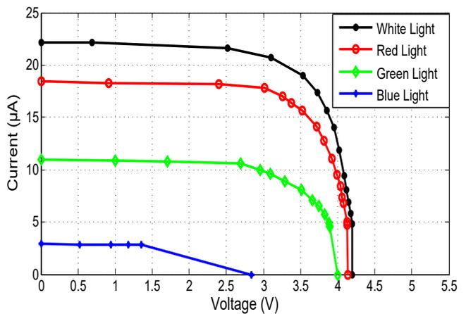
Figure 11: I-V Curves for different wavelengths of incident light
