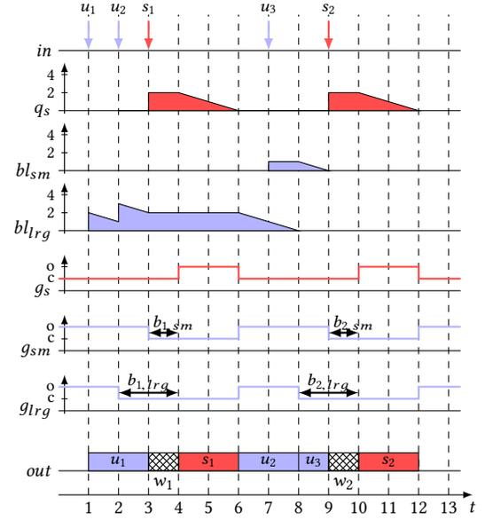
Figure 4: Bandwidth usage improvement with SBQ:  $len(u_1) = len(u_2) = len(s_1) = len(s_2) = 2$ ;  $len(u_3) = 1$
