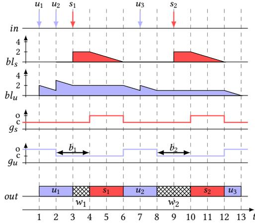
**Figure 2: Bandwidth usage inefficiencies caused by guard bands:**  $len(u_1) = len(u_2) = len(s_1) = len(s_2) = 2; len(u_3) = 1$
