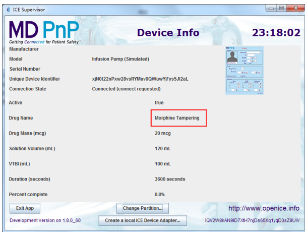
Figure 9: The tampered message displayed on the ICE Supervisor front panel.
